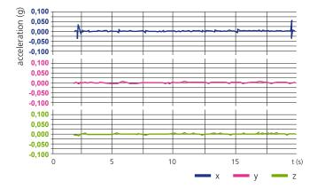
Vibrations of a test axis with roller guide and linear drive
